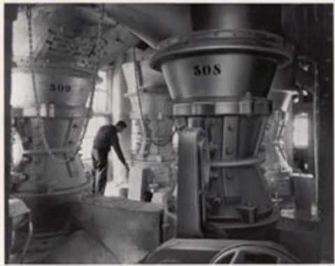
In the late 1930's, Sturtevant machines were used to crush and screen the salt.
